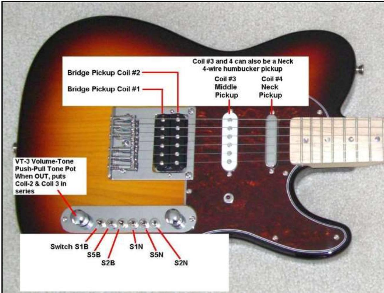
Here is how the mini-toggle controls of our T4-Switch and T4Plus-Switch product are laid out.
