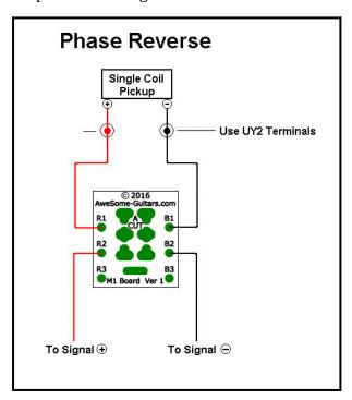
This example uses either a push-pull pot or a DPDT (On-none-On) mini toggle switch component to put two pickup coils into correct phase series.
