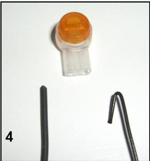
Figure 4 shows how to bend the 26 gauge wire ~ 5/16" (8mm) from non-stripped end. This is not necessary if you are using the UY2 connector to electrically join two 22 gauge wires.
