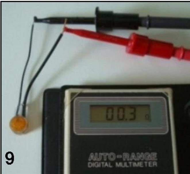
Figure 9 uses an ohmmeter to show electrical continuity connecting the two different gauge wires.
