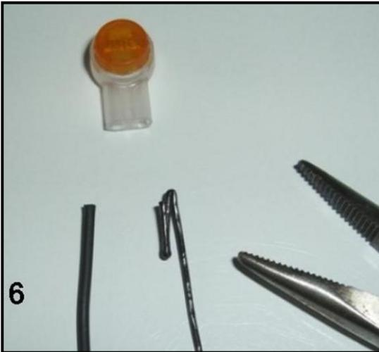
Figure 6 shows how to tightly crimp both wire bends with needle-nose pliers. This is not necessary if you are using the UY2 connector to electrically join two 22 gauge wires.
