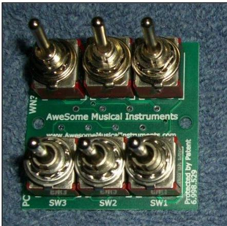
The **3-pickup version** uses six switches. Three of the switches are ON-OFF-ON and will go into the switch terminal pads labeled SW1, SW2 and SW3. Set these switches in the center (OFF) position. The other three switches are ON-ON and it goes into the switch terminal pad labeled SW4, SW5 and SW6. Set these switch paddles to face towards the center of the printed circuit board.
