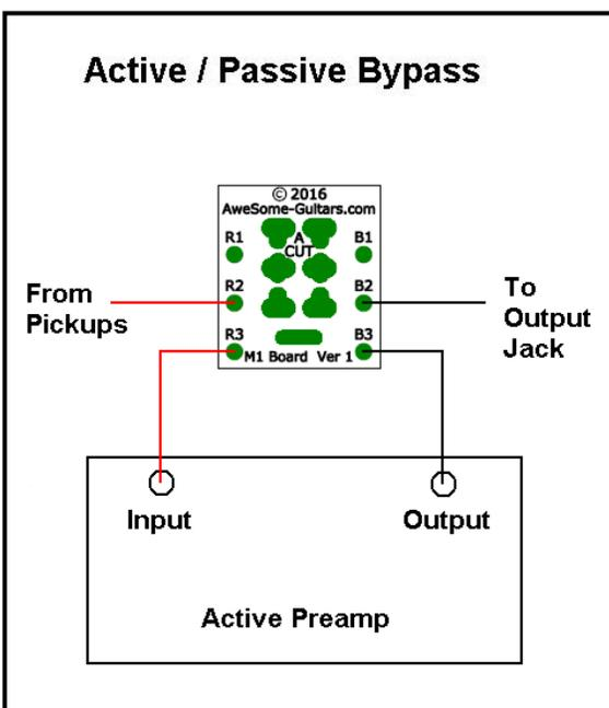
This example uses either a push-pull pot or a DPDT (On-none-On) mini toggle switch component to switch on or bypass an Active Preamp.
