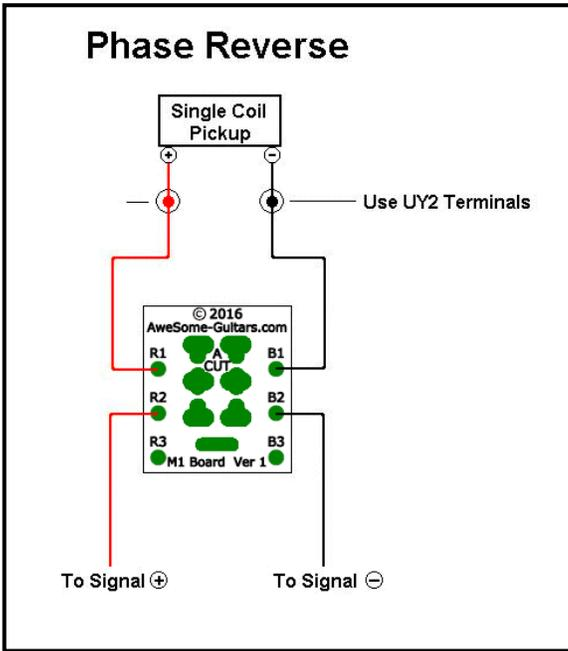
This example uses either a push-pull pot or a DPDT (On-none-On) mini toggle switch component to reverse the phase of a pickup coil. If a DPDT (On-Off-On) mini toggle switch is used, this lets you get both On-Off and phase switching control
