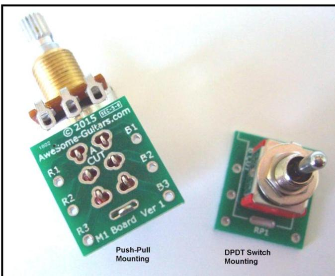
Examples of mounting a push-pull potentiometer and DPDT mini toggle switch to the M1-PCB.
